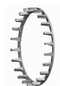
Fig. 7. YMD Split, machined-brass, land-riding, finger-type cage.
