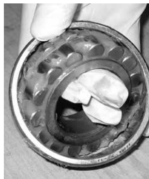
Fig. 21. Grease can easily be packed by hand.
