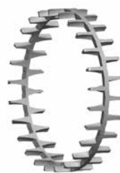
Fig. 5. EM/YM One-piece, machined-brass, roller-riding, finger-type cage.
